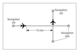
Figure 5-14. Ten-minute separation between aircraft on crossing tracks and same level (see 5.4.2.2.1.2 b))
