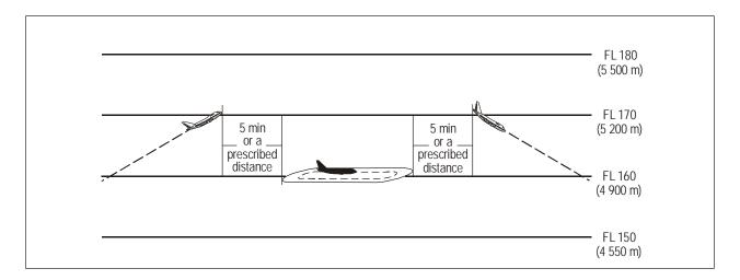
Figure 5-34. Separation between holding aircraft and en-route aircraft (see 5.5.2)
