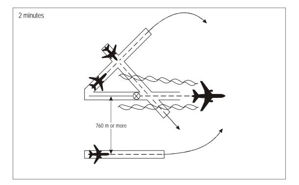
Figure 5-40. Two-minute wake turbulence separation for crossing aircraft (see 5.8.3.1 c) and d))
