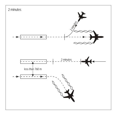
Figure 5-43. Two-minute wake turbulence separation for opposite-direction landing (see 5.8.5 b))
