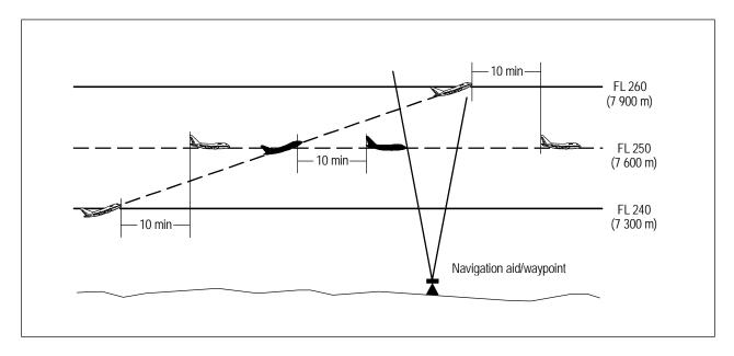
Figure 5-16A. Ten-minute separation between aircraft climbing and on same track (see 5.4.2.2.2.1 b))
