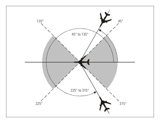
Figure 5-8. Aircraft on crossing tracks (see 5.4.2.1.5 c))
