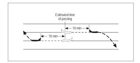
Figure 5-20. Ten-minute separation between aircraft on reciprocal tracks (see 5.4.2.2.3)
