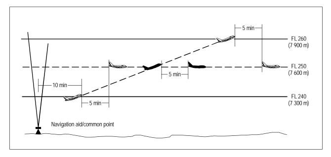
Figure 5-17A. Five-minute separation between aircraft climbing and on same track (see 5.4.2.2.2.1 c))
