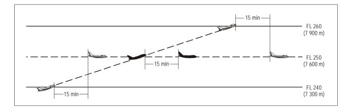
Figure 5-15A. Fifteen-minute separation between aircraft climbing and on same track (see 5.4.2.2.2.1 a))
