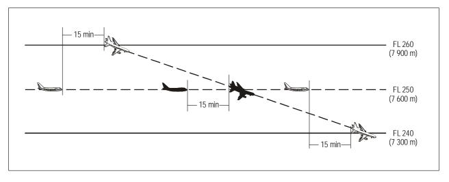
Figure 5-18B. Fifteen-minute separation between aircraft descending and on crossing tracks (see 5.4.2.2.2.2 a))
