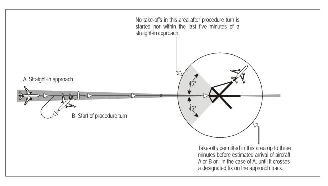
Figure 5-38. Separation of departing aircraft from arriving aircraft (see 5.7.1.1 b) and 5.7.1.2 b))
