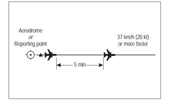
Figure 5-11. Five-minute separation between aircraft on same track and same level (see 5.4.2.2.1.1 c))
