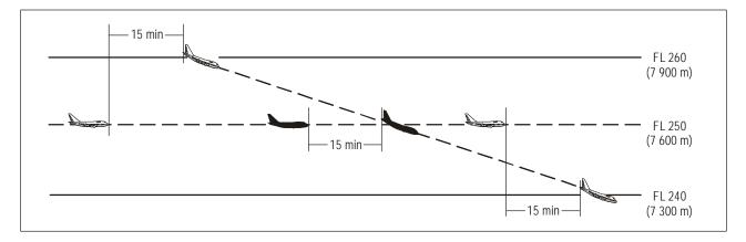
Figure 5-15B. Fifteen-minute separation between aircraft descending and on same track (see 5.4.2.2.2.1 a))
