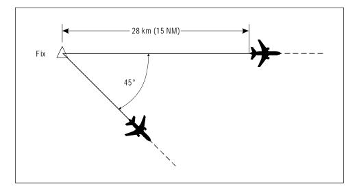
Figure 5-4. Separation using dead reckoning (see 5.4.1.2.1.2 c))
