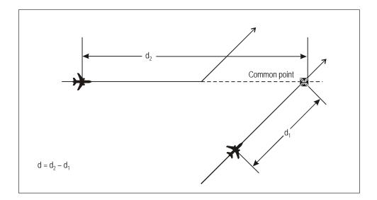
Figure 5-31. Calculation of longitudinal distance between aircraft — same track projected, but not identical (see 5.4.2.6.4.1 b))
